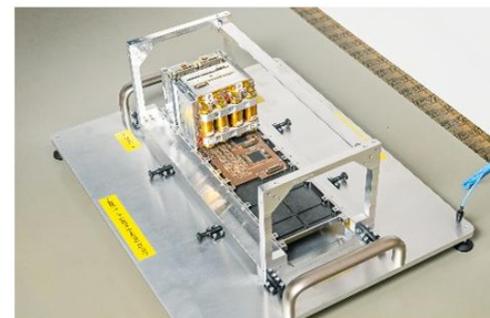
Figure 6.5: C3S 3U CubeSat Structure. Credit: Complex Systems & Small Satellites.
