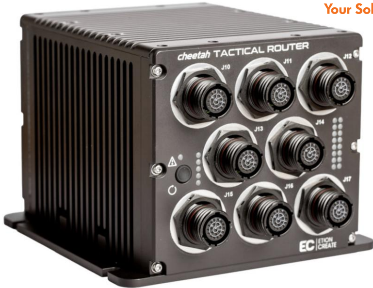
Figure 4: Cheetah Tactical Router in rugged VNX+ format (Figure: Sundance)
