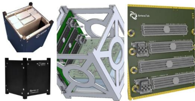
[Figure 7 | Pictured is a 1U CubeSat with SpaceVNX modules. Photos: Trident-Infosol, Ideas-Tek, Antara Teknik.]
