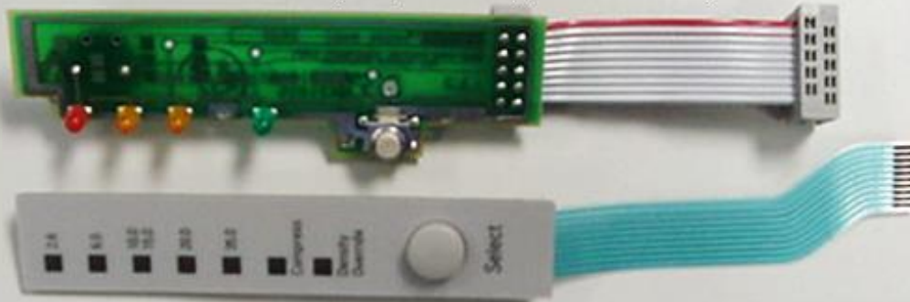
Previous Construction (PCB, Cable Assy, Soldered LEDs)
