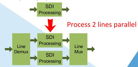
Selected system clock 135 MHz (→270 MHz @ 20-bits)
