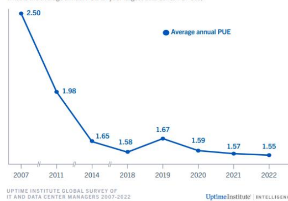
What is the average annual PUE for your largest data center? (n=669)
