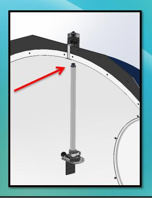
4Pi post will have a built in electrical connector. The mating connector will be hardwired into each of the two mounting blocks. This will allow the post to simply 'plug' into the mounting block and eliminate feeding banana plugs through the block along with bundles of wire.
