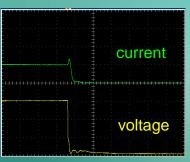
10uS spike duration 30% over current One device failure
