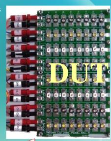
Models from 50V-400V, 10mA-64A DC, Pulsed current Individual current control Up to 120 3V LEDs/channel, 960 LEDs/module, 30,720 LEDs/system
