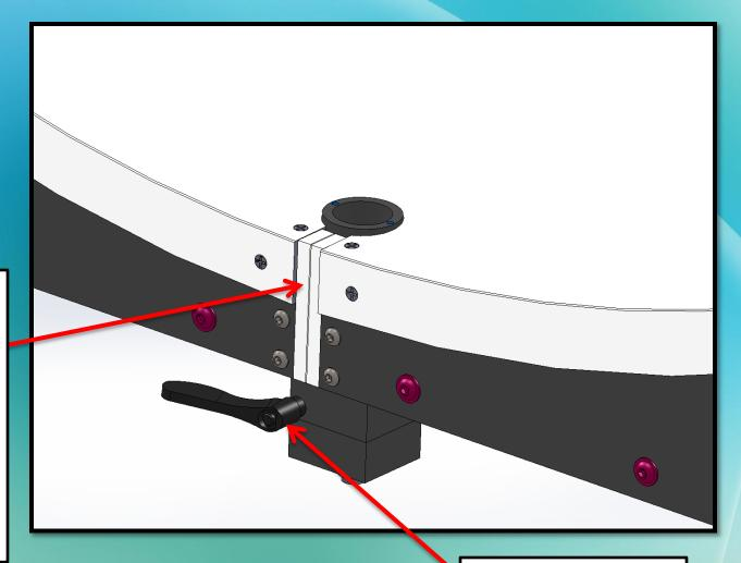
Adjustment Lever allows installing 4Pi post to be done tool free
