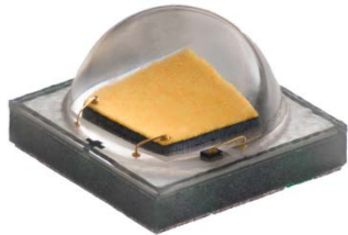
High power led Cree 3.5 x 3.5mm Max 4W
