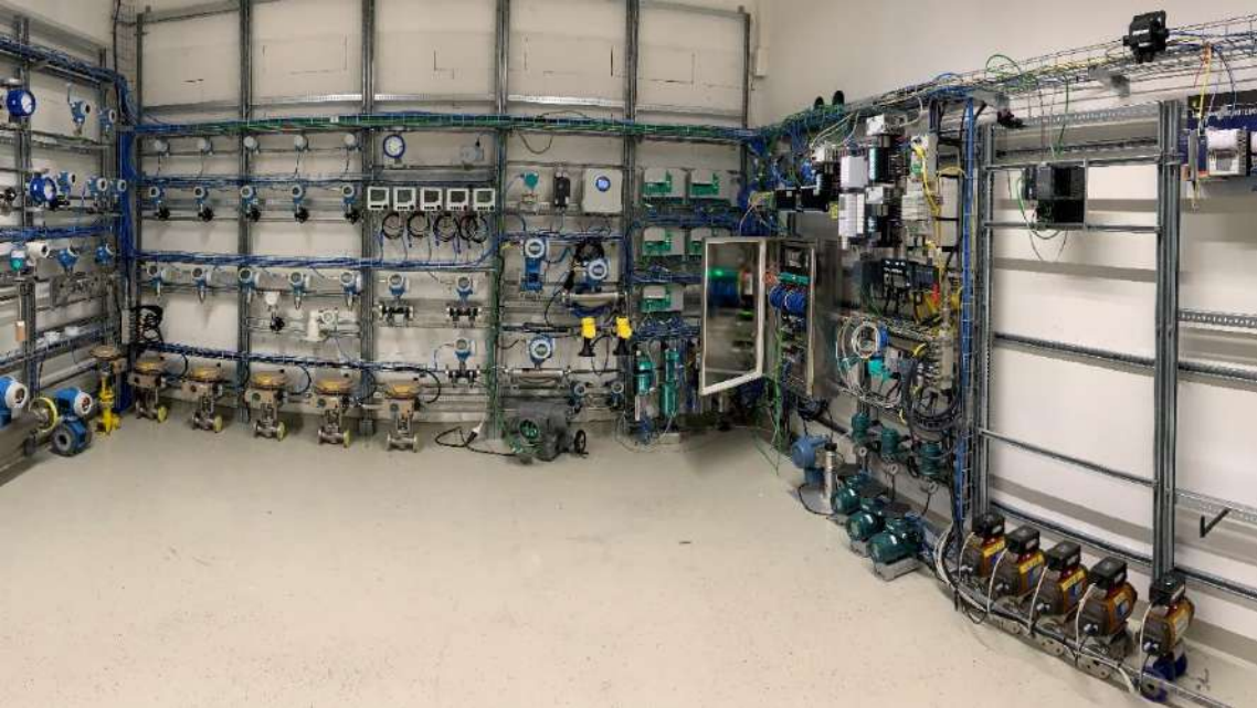
Field Level with sensors and actuators
