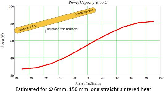
Estimated for  $\phi$  6mm, 150 mm long straight sintered heat pipe at 50  $^{\circ}{\rm C}$
