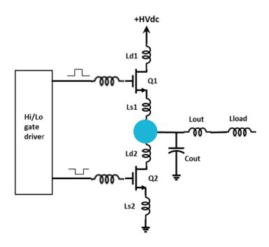
Probing to floating point with shorted differential probe
