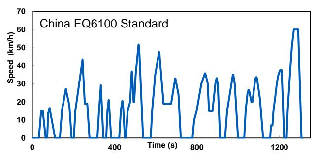
Maximum speed = 62 km/hAverage speed = 16.5 km/hAverage acceleration =  $0.39 \text{m/s}^2$ Average braking =  $-0.48 \text{m/s}^2$ . Total distance = 6 km. Duration = 1314 secIdle time: 373 sec, (28.4%)
