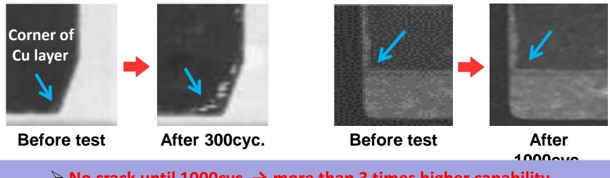
$\blacktriangleright$  No crack until 1000cyc.  $\rightarrow$  more than 3 times higher capability
