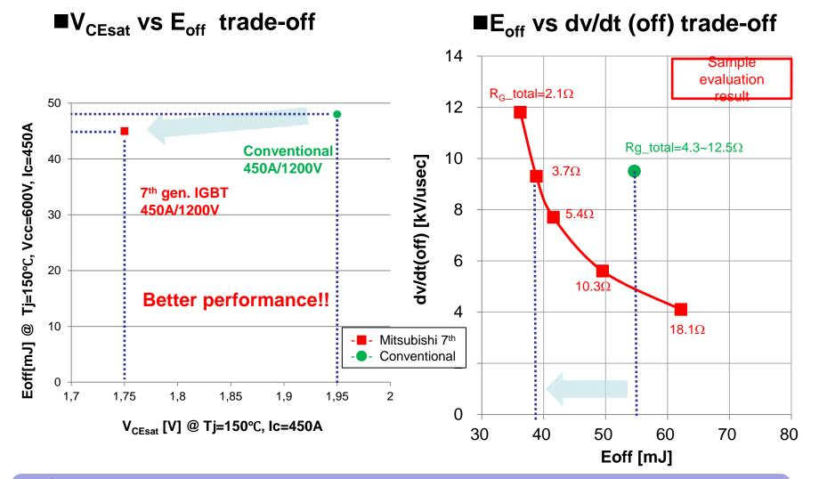
7<sup>th</sup> gen. IGBT has better static and dynamic characteristics. It also has better controllability of dv/dt with R<sub>G</sub>.
