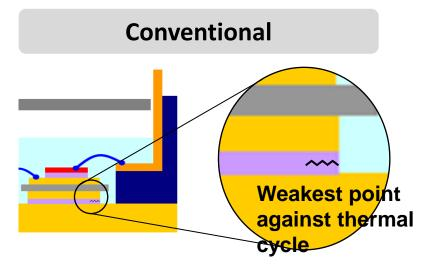
Temperature cycling test (-40°C ~ 125°C)
