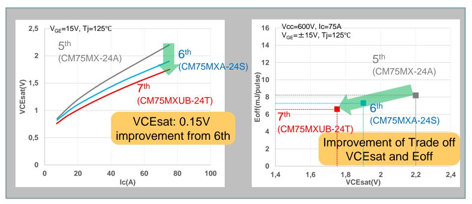
**Power loss is reduced with 7th-Gen. IGBT**
