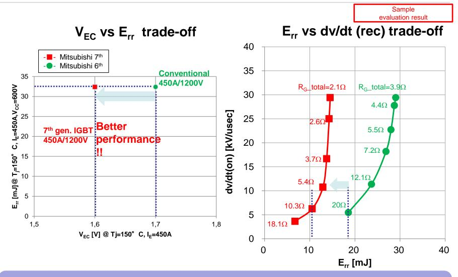
RFC diode improves the  $E_{rr}$  vs.  $V_{EC}$  trade-off from 6<sup>th</sup> gen. Diode. Err against dv/dt is further reduced than the other diodes.
