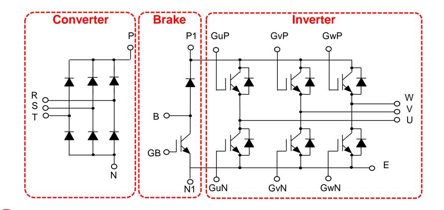
Smaller, simpler design for inverter systems
