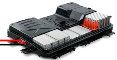
E-Vehicle battery 384V 180Ah 69.12kW
