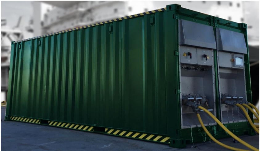
Battery Container Swapping Solution (Source: Bakker Sliedrecht)
