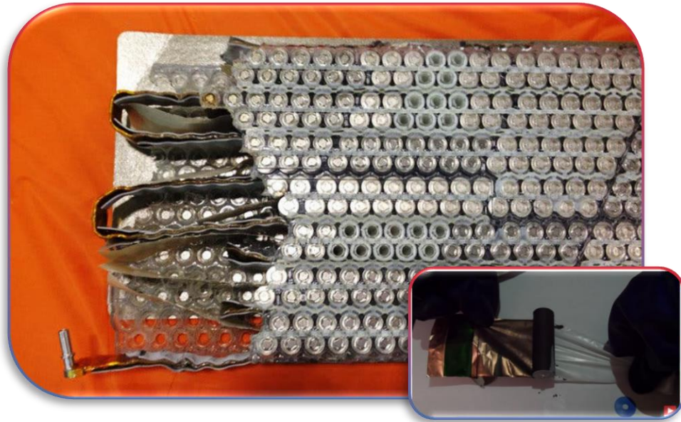
Tesla 3 Battery Pack & 2170 cell interior (ARES RC Youtube Channel)
