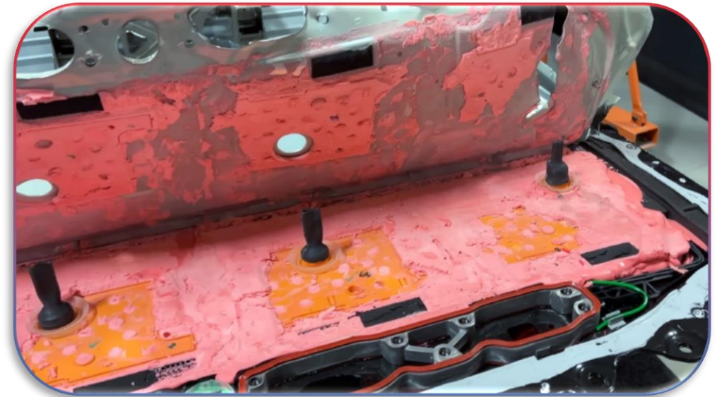
Tesla Y Battery Pack & 4680 cell interior (Munro Youtube Channel)
