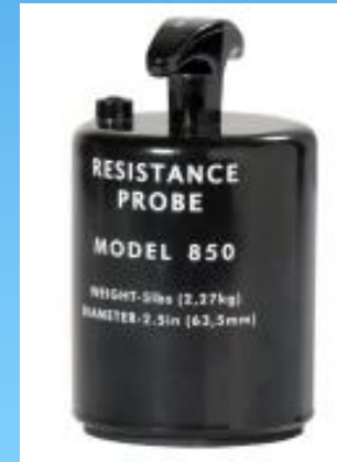
Probe acc. to IEC61340-4-1
