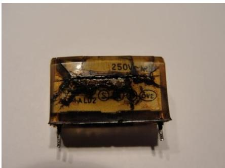
Increased current destroys capacitors, and increases Earth current (causing protection problems, and possible safety issues).
