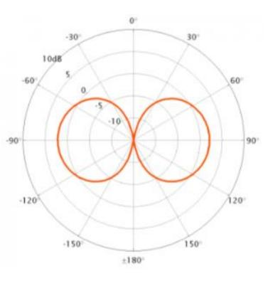
Specification from SCAN antenna: <u>http://www.scan-antenna.com/product/vhf0hd-0-</u> <u>db</u> VHF0HD 0 dB Heavy-duty end-fed full 1/2  $\lambda$ dipole marine antenna
