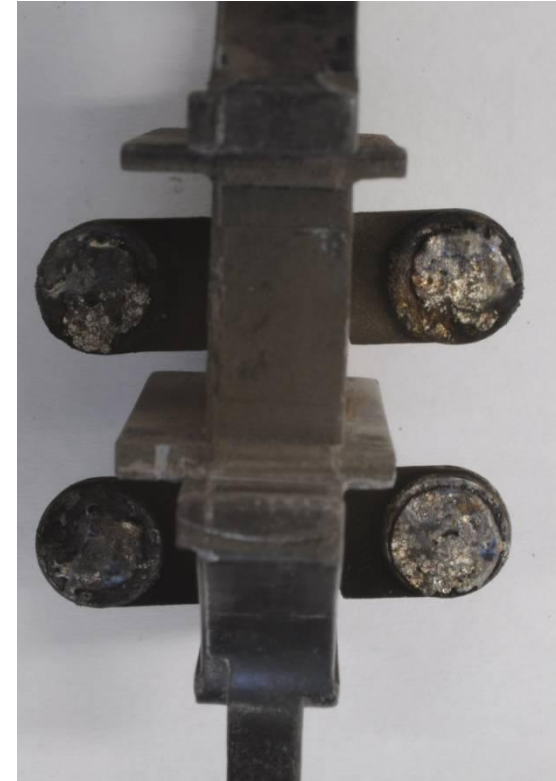
After about 3 years (note: one contact broken off due to melting of support piece)
