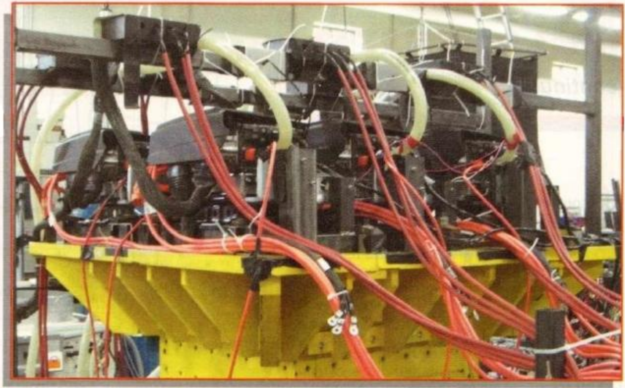
FIG. 1 – RFMPT setup for an automotive power electronics unit.
