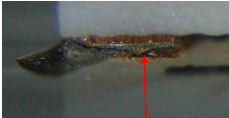
Crack in 2 nd level solder joint HB-LED
