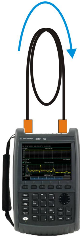
2-Port 'Transmission' Loss Measurement
