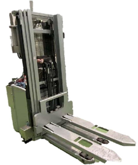
Forklift in cardboard manufacturer Batteries + DC converter
