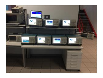
Seven RSA5000B's on an Elabo bench, showing views in DPX mode to discover illusive signals, and demodulation analysis screens to look 'into' the signals. On the top row, a new RSA306 USB PC/laptop driven spectrum analyzer can be seen.
