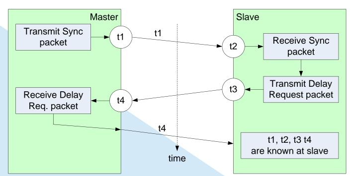
network delay = t2 - t1 - (offset between master and slave) network delay = t4 - t3 + (offset between master and slave) Offset between master and slave = (t2 - t1 - t4 + t3) / 2
