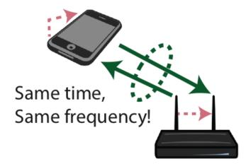
• TX and RX *simultaneously* at *same* frequency
