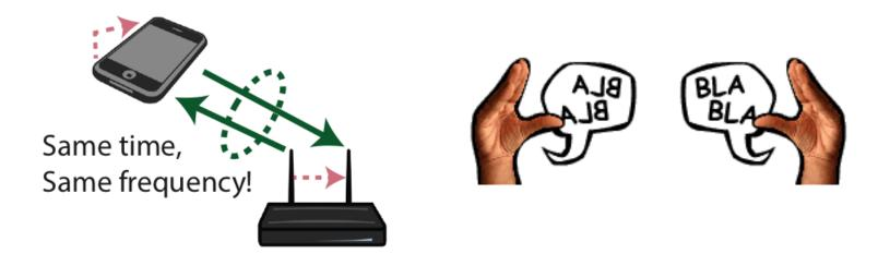
• TX and RX simultaneously at same frequency
