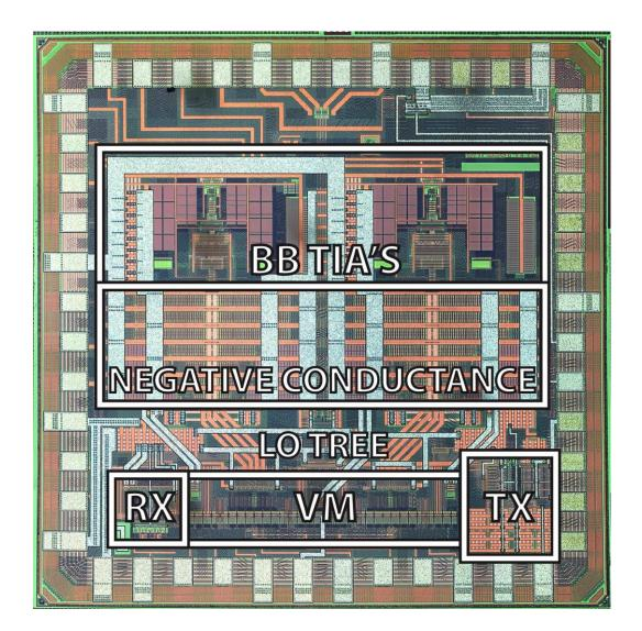
65nm CMOS 1.2V supply 1.4x1.4mm
