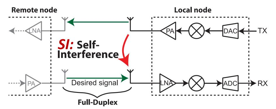
• P<sub>TX</sub>: ~0..20dBm RX-Sensitivity: ~-100..-70dBm
