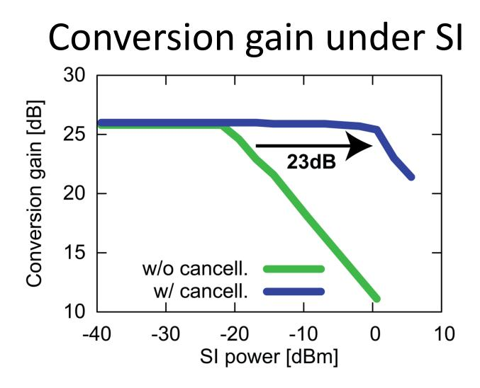
Desired signal only compressed at >0 dBm SI = 20dBm TX power at 20dB iso
