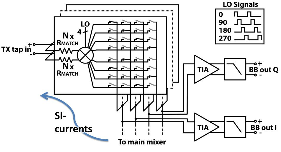
SI diverted through passive networks (extreme linearity)
