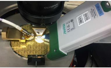
Even connect the MS2760A directly to a wafer probe!
