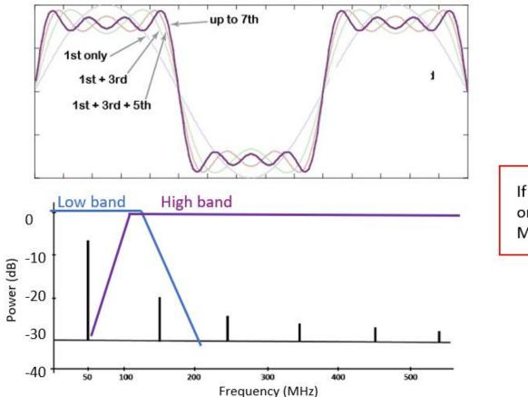
If band switching is used, or system bandwidth is poor, Measurement errors occur!
