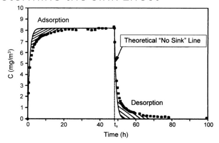
In a good chamber the theoretical curve and the measured curve are nearly equal.
