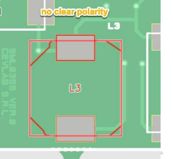
No polarity indication between Component Placement List and Gerber data
