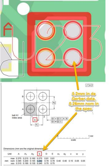
Component specs not respected in the PCB layout
