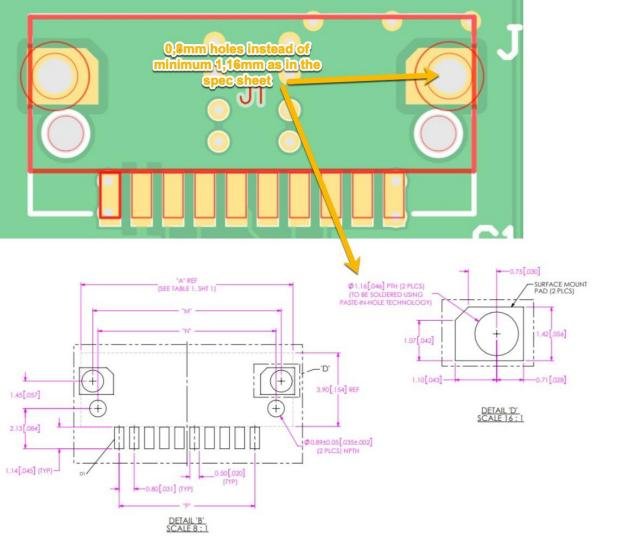
Component specs not respected in the PCB layout
