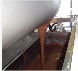
2. Mixing unit on top of the molds for adding liquid additives, nuts, raisins etc.
