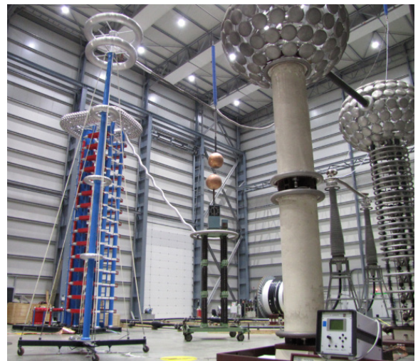
Figure 6. High voltage equipment for AC (left) and DC (right) cable testing at KEMA Labs.
